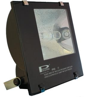
Die cast aluminium floodlight sealed to IP65 with toughened glass front retained by hinged stainless steel clips. Galvanised steel stirrup type mounting bracket supplied. Two sizes of body available for the full range of wattages in SON and HQI from 150w to 400W. Can be produced in either Asymmetric or Symmetric versions. Wall or column mounted, stirrup bracket allows for 180 degree movement. Integral photocell option available.
